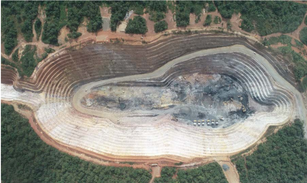
Figure 2: Namakan Pit at Tabakoroni (completion of Stage 2 cutback with pit floor at Stage 1 level)
