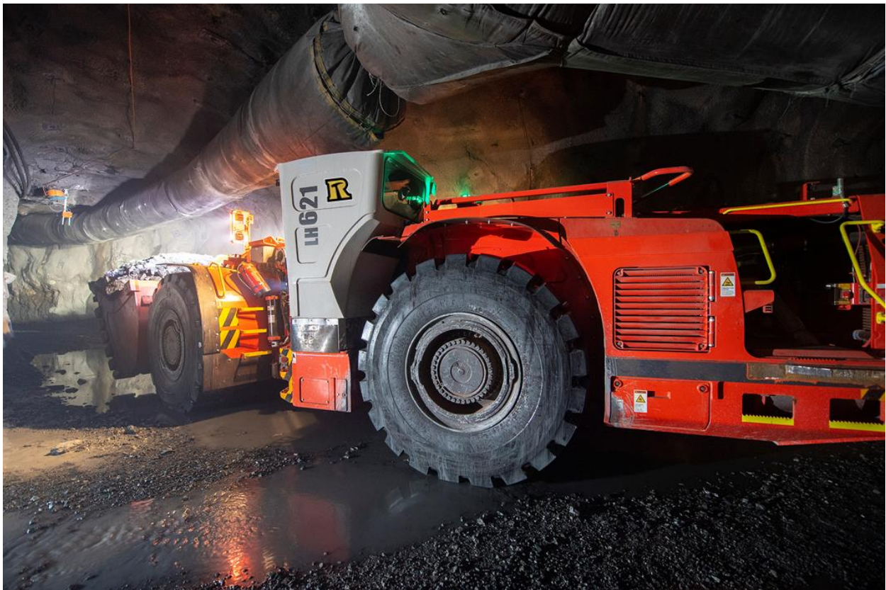
Figure 6: Autonomous primary loader hauling ore from the 1105 level
