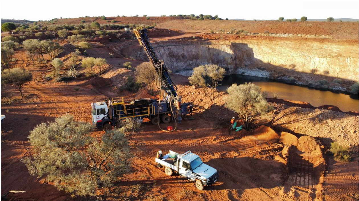
Figure 2: RC drilling commencing at the Eagle Prospect
