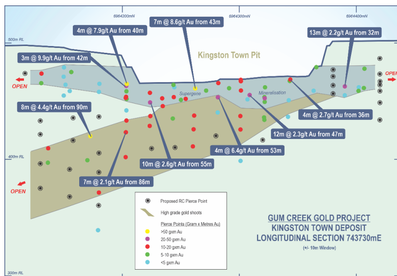
Figure 8: Kingston Town long section showing gold gram x metre pierce points (>25 Au gram x metres labelled), historic open pit supergene mineralisation, interpreted high-grade ore shoots, and current drill program mineralisation pierce points
