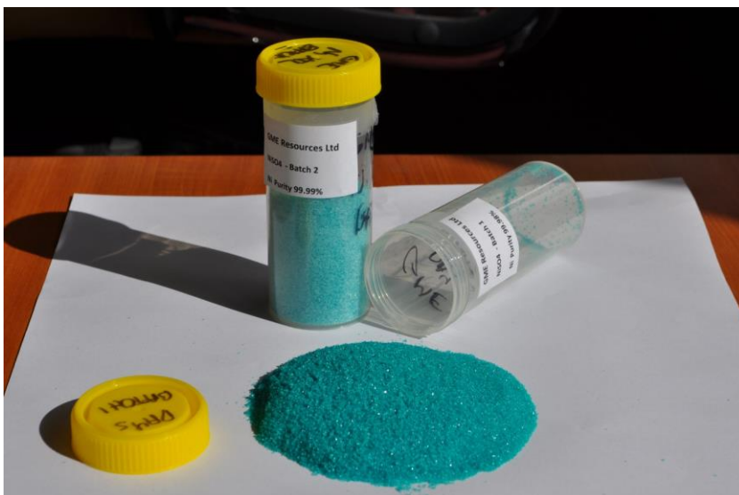
Figure 5: Nickel sulphate produced from NiWest ore through GME’s metallurgical test work program
