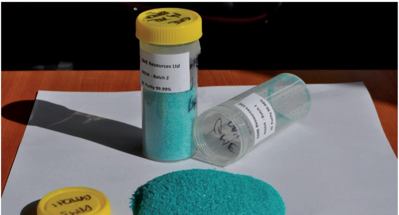
Figure 6: Nickel sulphate produced from NiWest ore through GME's metallurgical test work program
