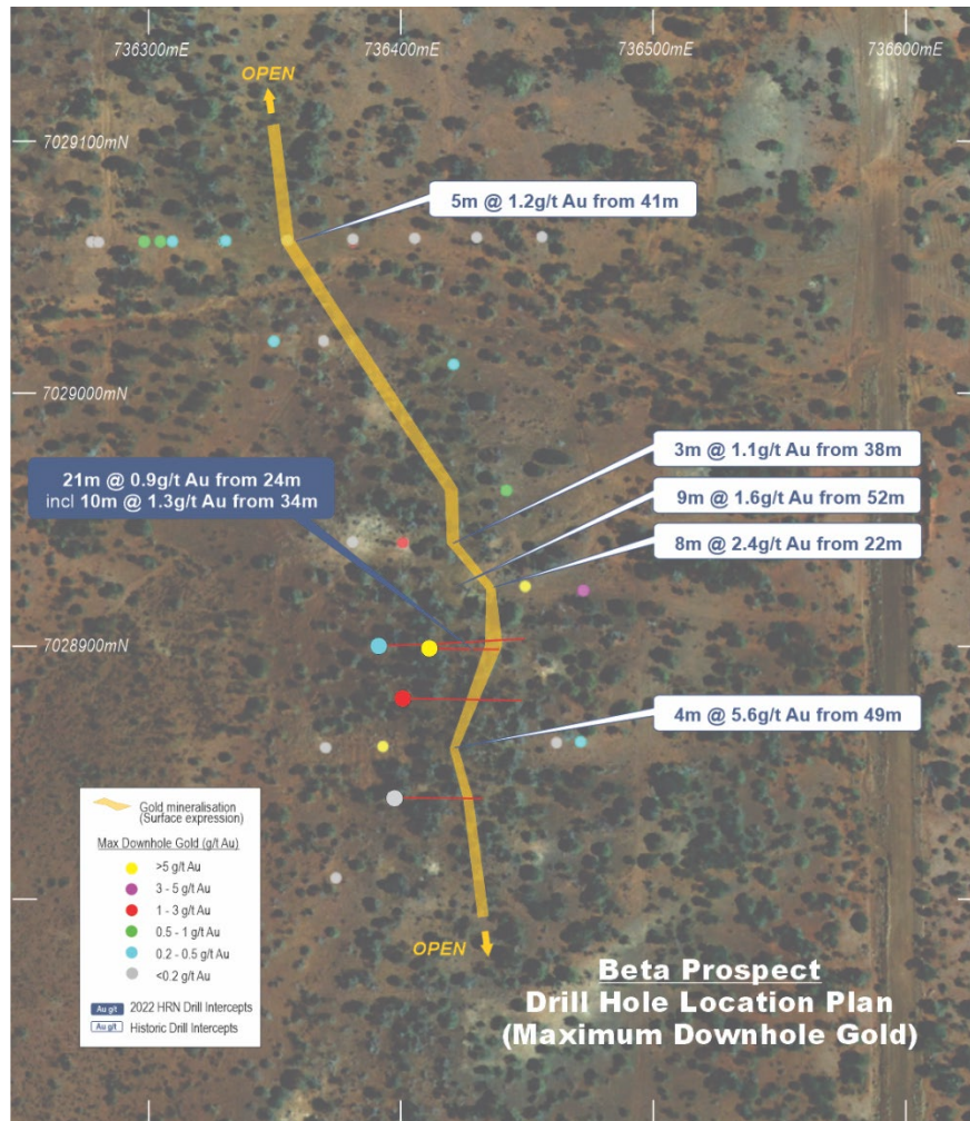
Figure 20: Beta drill hole plan showing all collars coloured by maximum downhole gold with all drilling intercepts (>3 GxM) labelled over satellite image.
