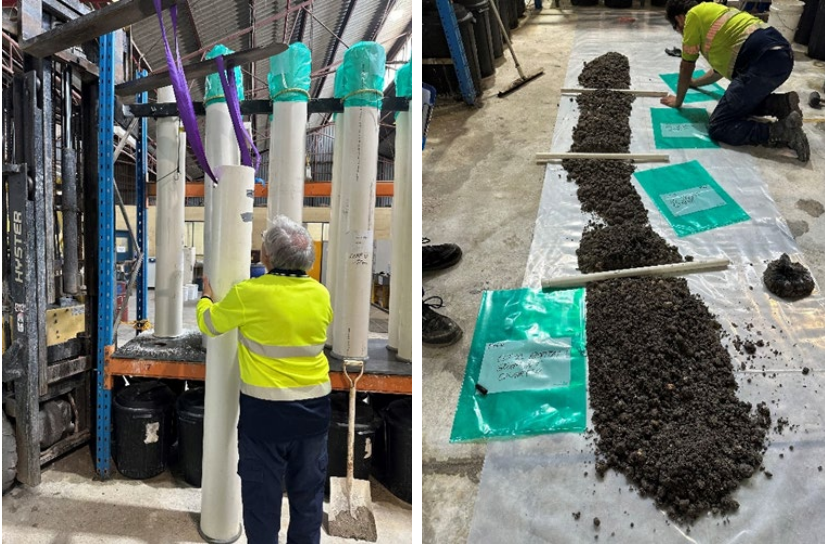
Figure 1 and 2: Completed columns being disassembled from column leaching workframe
