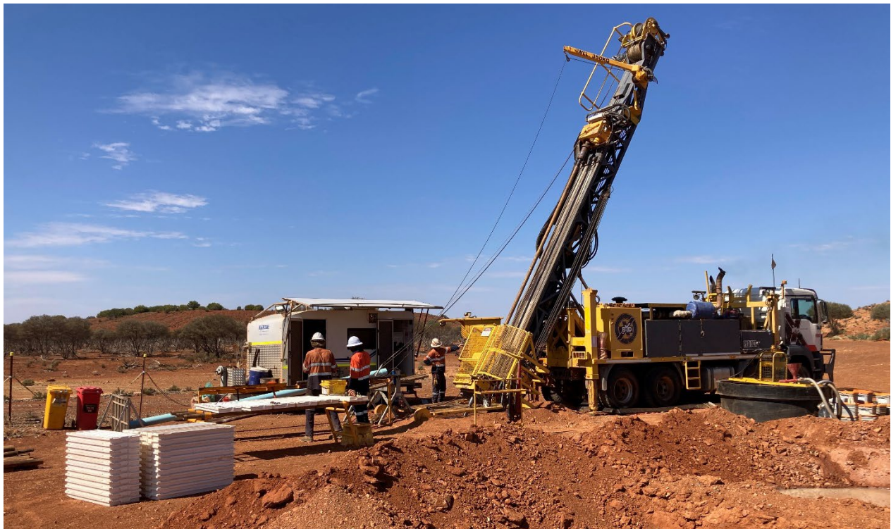
Figure 2: Diamond drilling at the Wedge Prospect.
