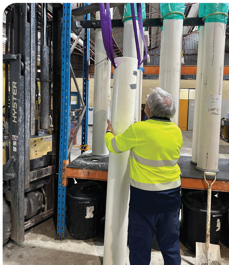
Figure 6: Completed columns being disassembled from column leaching workframe
