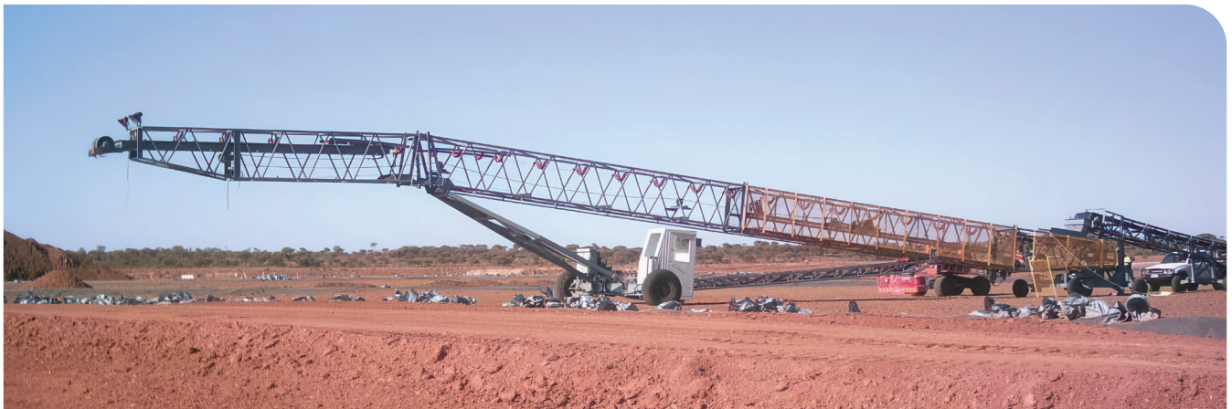
Figure 7: Heap leach conveyor stacker example
