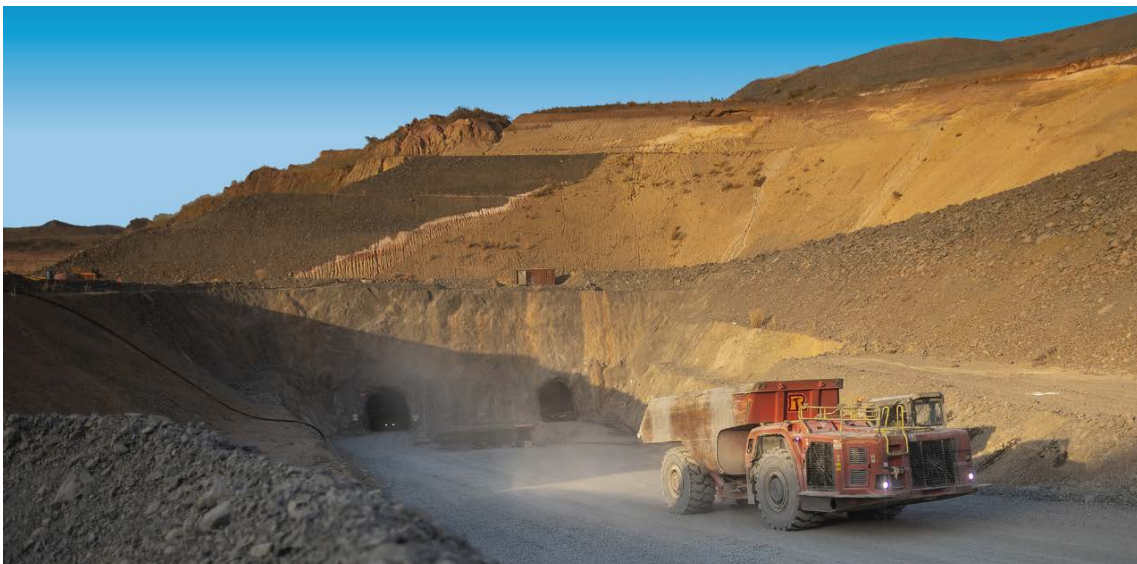
Figure 1: Automated Haul Truck leaving the Syama Underground Mine Portal
