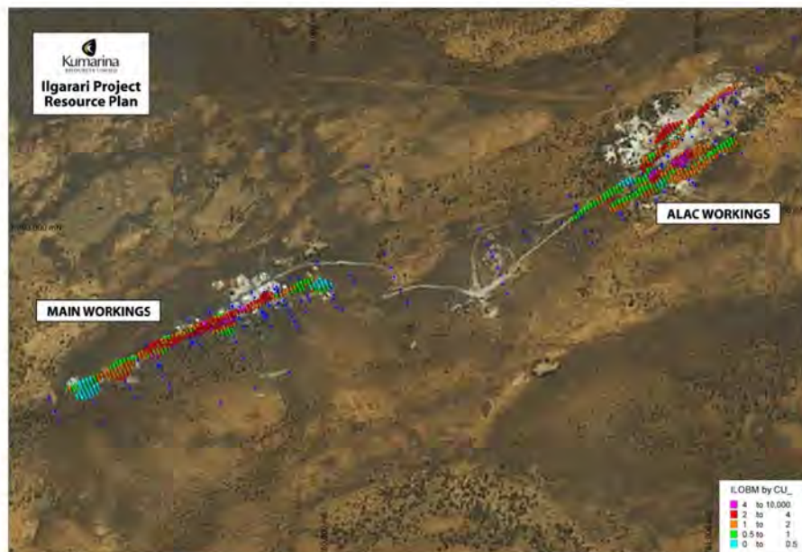
Figure 11: Plan View of The Block Models For The Main and Alac Zones
