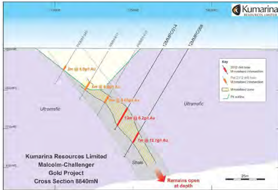
Figure 17: Malcolm-Challenger Gold Project Cross Section 8840mN
